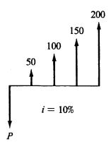
5-2 Compute the value of P that is equivalent to the four cash flows in the diagram below.
