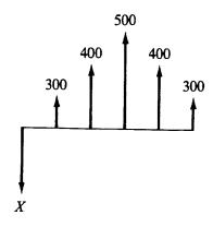
**4-11** Compute the value of P in the diagram below using a 15% interest rate.
